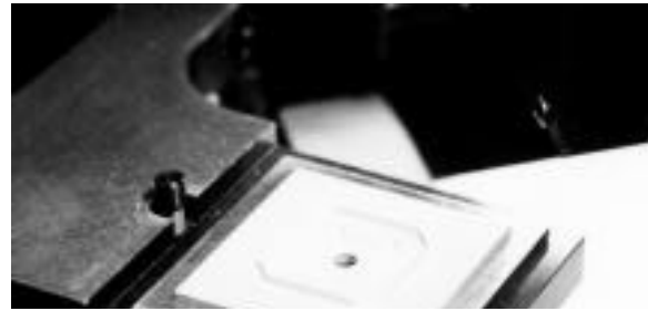
Component Reflex Register. This swings under the VPD so that the DABIS vacuum pickup can “capture” the component and place it on the PCB.
