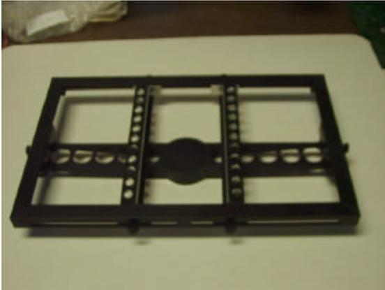
The standard adjustable circuit Board Holder can accommodate boards up to 12" wide. Most PCBs will be smaller. The Board Holder consists basically of two supports with adjustable edge-holding fingers. Both supports can slide back and forth across the adjustment bars, and can be fixed in position by tightening black-knobbed friction screws as shown in the illustration.
